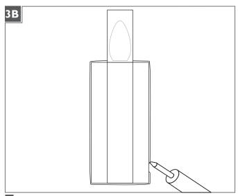
**For wet locations**, caulk around the base with waterproof construction sealant.
