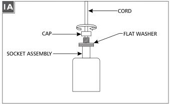
Unscrew fixture cap and remove the cap and top flat washer from the socket assembly and cord.
