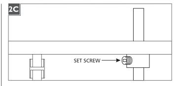
Loosen (**Do Not Remove**) the set screw on the strain relief.
