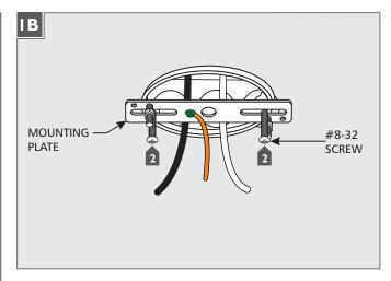
2 Mount the mounting plate assembly to the electrical box with the two provided #8-32 screws.
