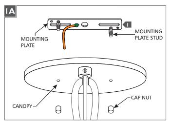
Remove the mounting plate from the canopy by unscrewing the cap nuts from the mounting plate studs.
