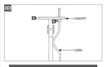
NOTE: The power cord does not support the fixture. For a casual "lazy cord" look, cut the power cord several inches longer that the drop height of the fixture.
