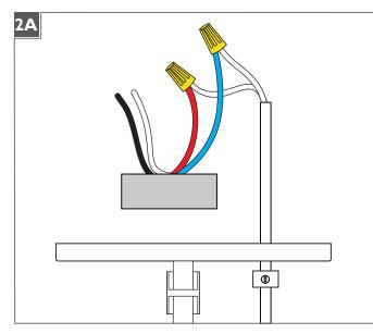
Take note of the wire connections and remove the wire nuts to disconnect the power cord wires from the driver wires.
