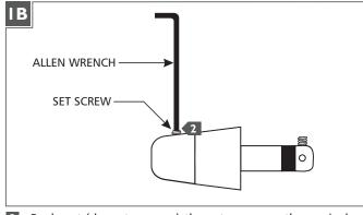
**2** Back out (do not remove) the set screw on the conical connector with the provided Allen wrench.
