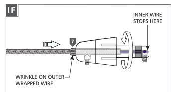
Keep pushing the coaxial cable into the connector while rotating the connector to ease feeding the inner wire into the tip of the connector. The outer wrapped wire will start wrinkling while being inserted another 1/2" into the connector.
