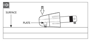
5 Tap the conical connector on a hard surface with the set screw facing down, so the plate inside drops into place.
