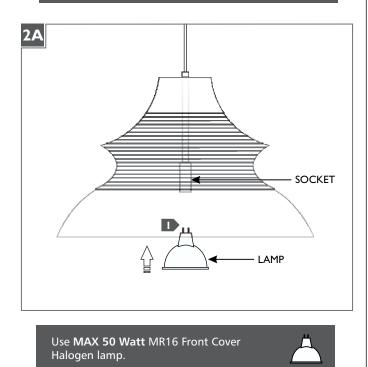
Push the lamp pins completely into the socket holes.
