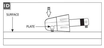
Tap the conical connector on a hard surface with the set screw facing down, so the plate inside drops into place.
