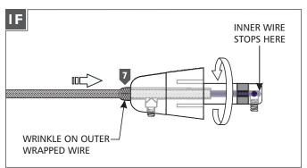
7 Keep pushing the coaxial cable into the connector while rotating the connector to ease feeding the inner wire into the tip of the connector. The outer wrapped wire will start wrinkling while being inserted another 1/2" into the connector.
