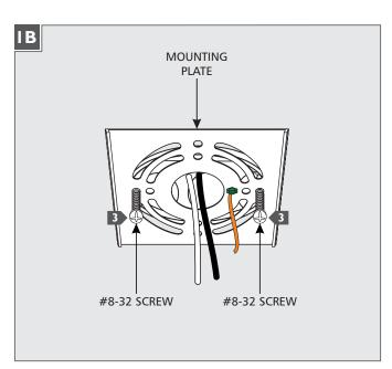
Attach the mounting plate to the electrical box using the two #8-32 screws provided.
