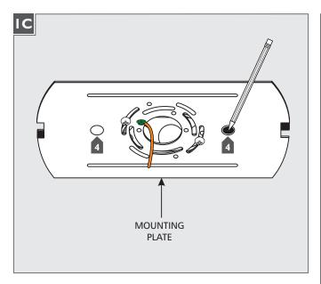
4 Mark the two anchor locations and uninstall the mounting plate from the electrical box.
