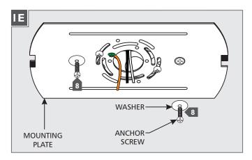
Secure the mounting plate to the anchors with the washers and anchor screws.
