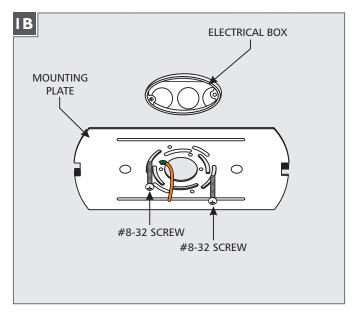
For Tenur 10 Only: Secure the mounting plate to the electrical box with the two #8-32 screws. Skip to step 1F.
