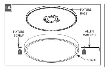
Separate the fixture base from the shade by unscrewing and removing the three fixture screws using an Allen wrench.
