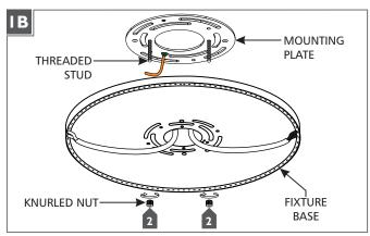
Remove the mounting plate from the fixture base by unscrewing the two knurled nuts from the two threaded studs.
