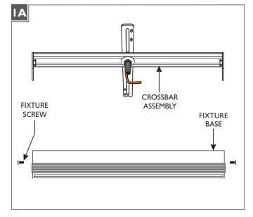
Separate the crossbar assembly from the fixture base by unscrewing and removing the two fixture screws.
