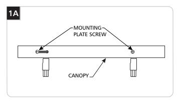
1 Separate the mounting plate from the canopy by removing all four screws.
