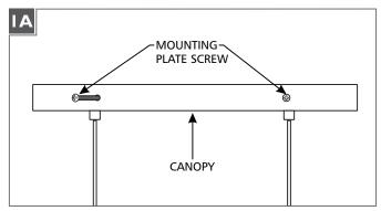
Separate the mounting plate from the canopy by removing all four mounting plate screws with a screw driver.
