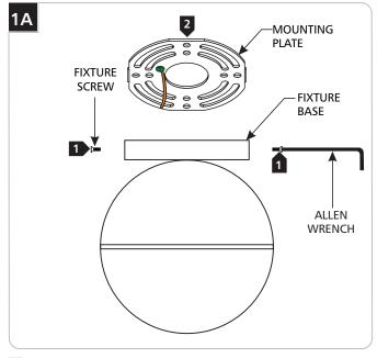
1 Remove the fixture screws located on both sides of the fixture base using the provided Allen wrench.
