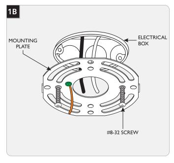
Mount the mounting plate to the electrical box using the provided #8-32 screws.
