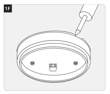
**9** For wet location installation, caulk around the fixture base with waterproof construction sealant.
