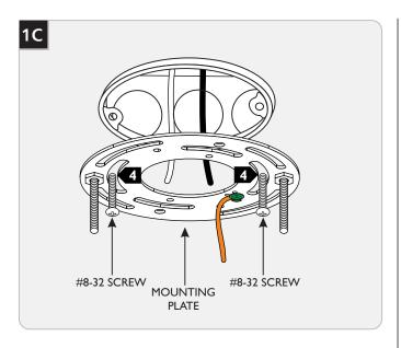
Install the mounting plate to the electrical box with the two #8-32 screws.
