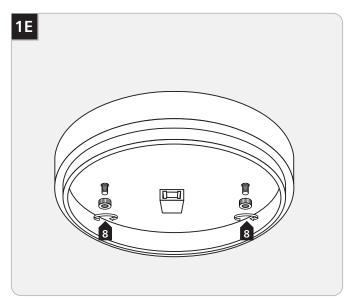
Mount the fixture base to the ceiling by reinstalling it onto the mounting plate and securing it tightly with the knurled nuts.
