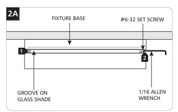
Place the glass shade into the fixture base until the grooved section of the glass shade is completely inside.
