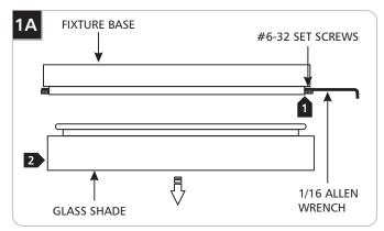
While supporting the glass shade, loosen (Do Not Remove) the four #6-32 set screws on fixture base with the 1/16 Allen wrench.
