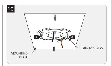
Secure the mounting plate to the electrical box with 2 #8-32 screws.
