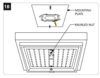
Remove the mounting plate from the fixture base by unscrewing the two knurled nuts.
