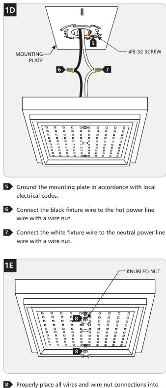
Properly place all wires and wire nut connections into the electrical box, mount the fixture base to the ceiling by reinstalling it onto the mounting plate, and secure it tightly with the knurled nuts.
