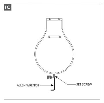
With the Allen wrench provided, back out (do not fully remove) the set screw at the base of the fixture.
