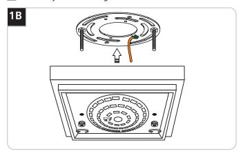
Remove the mounting plate from the fixture base by unscrewing the two knurled nuts.
