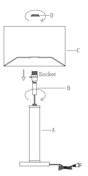
1. Screw socket part(B) clockwise onto part(A) to tighten.
